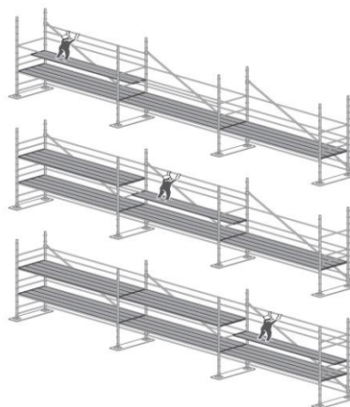
Figure 3: Erecting a Scaffold
